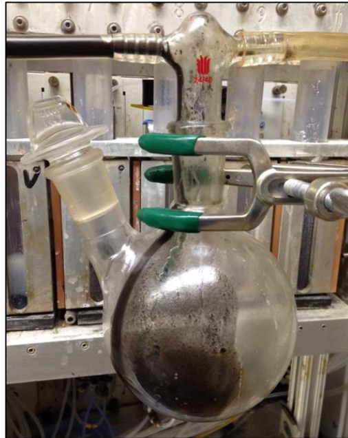
Figure 8.2: Photo of round bottom flask used in the continuous flow synthesis of FeCo/cobalt ferrite product with input tube (left) shown carrying synthesized nanomaterial to a holding vessel with the second tube (right) generating the partial vacuum.
