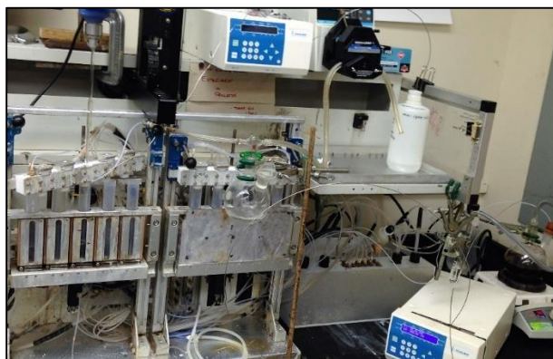
Figure 8.1: Photo of the involved continuous flow (CF) reactor set-up shown with systolic and peristaltic pumps (top), mechanical stirrer (top-left), reaction vessel (far left-center) and product vessel/round bottom flask (left-center).
